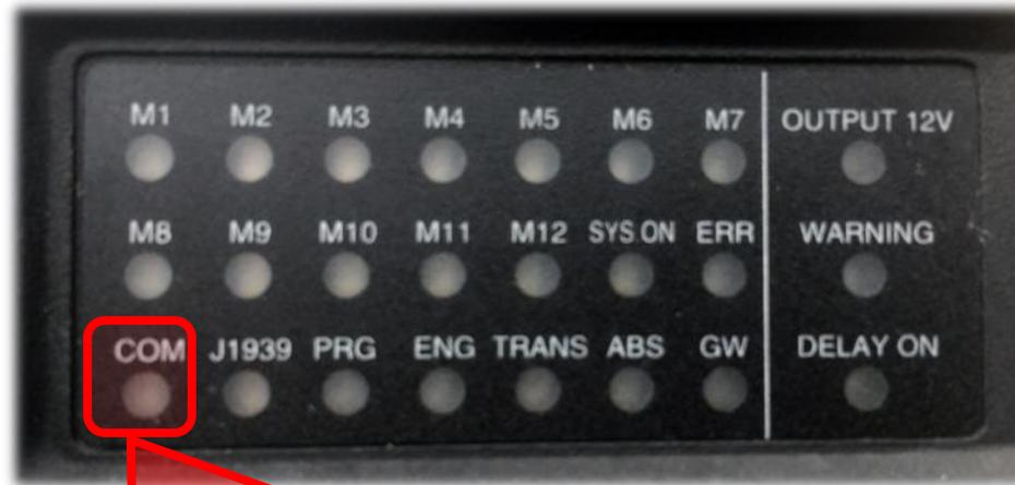
**COM Status:** The COM indicator flashes when the MBC program is transmitting and receiving data over the DINEX network.
